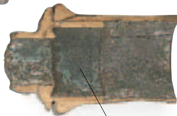
This section has been cut away to reveal the outlet valves and to show the carefully made pipe-joints
